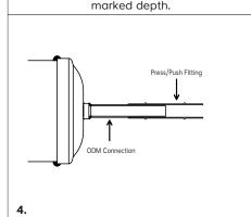
Push the tubes into the Press/Push fittings at both sides of the Filter Drier until they reach the marked depth.
