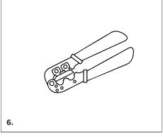
Activate the Press/Push tool to compress the fittings, securing the joints between the refrigerant lines and the Filter Drier.
