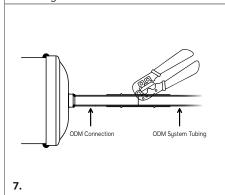
Ensure the tubes are fully inserted and the connections are properly compressed around the Filter Drier and refrigerant lines.
