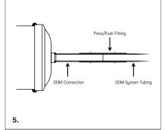
Adjust and position the Press/Push tool according to the fitting size for both the refrigerant lines and Filter Drier.
