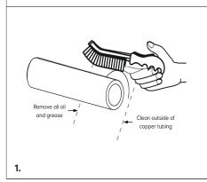
Deburr and clean the inside and outside of the tube ends.
