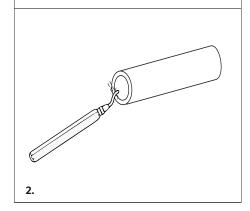
Mark the insertion depth on the tube end & the Filter Drier connections for correct engagement.
