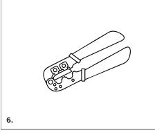
Activate the Press/Push tool to compress the fittings, securing the joints between the refrigerant lines and the Filter Drier.
